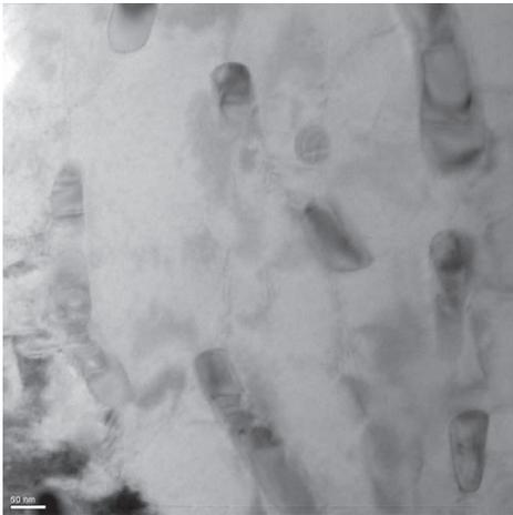
**Fig. 8.** Wire-like particles consisting of an outer wall partly filled with a dense material. TEM image of a preliminary study of sabre No. 9 (according to Zschokke [7]) showing similar nanostructuring like sabre No. 10
