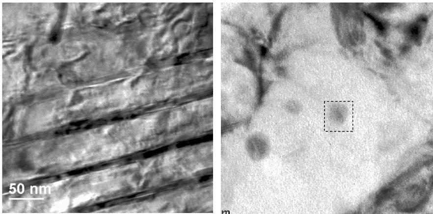
**Fig. 1.** TEM image of cementite nanowires in a Damascus sabre. Left panel: The dark stripes indicate wires of several hundreds nanometers in length. Right panel: View showing an almost circular cross section (dotted)
