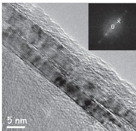
**Fig. 5.** Straight homogeneous remnant with a fringe spacing of 0.342 nm, which is characteristic of carbon nanotubes, in this case multiwalled
